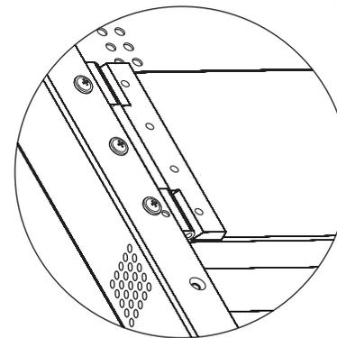
Attach the C-1332 to the left extension piece using the screws provided.
