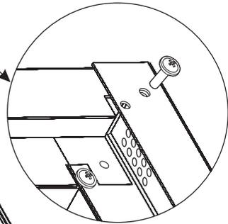
**Note: The top and bottom sections of the C-1355 have mounting holes for the optional C-1334 fan kit.**
