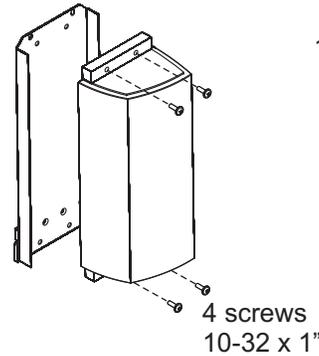
1. Attach the Bose® amplifier to the back side of the C-1332 Hinged Mounting Plate.
